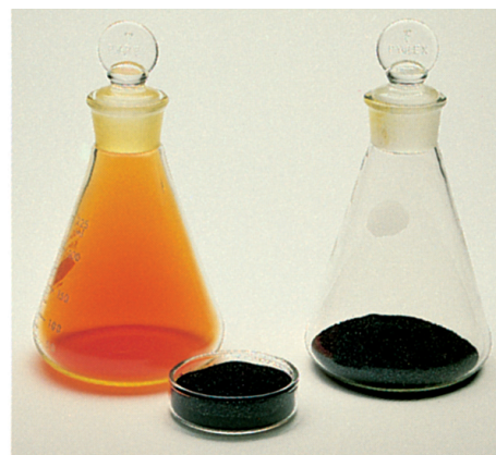
Figure M.3 The flask on the left contains nitrogen dioxide, \text{NO}_2(g) , and the dish in front contains activated carbon, a black powder. The flask on the right shows the result of adding the activated carbon to the flask containing \text{NO}_2(g) . Observe that the \text{NO}_2(g) has been completely absorbed.
