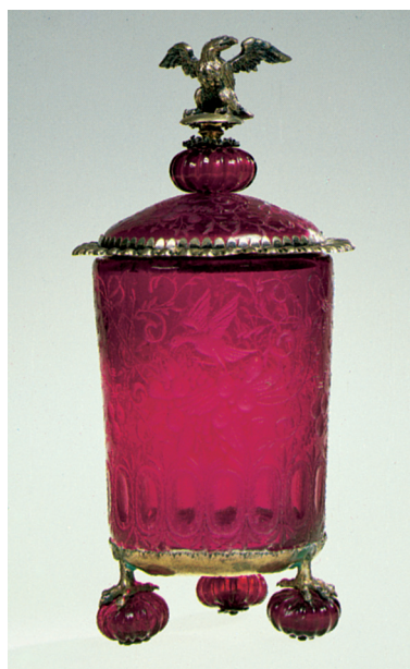
Figure M.15 A decorative container made of ruby glass. The rich red color of ruby glass is due to a dispersion of very finely divided gold throughout the glass.
