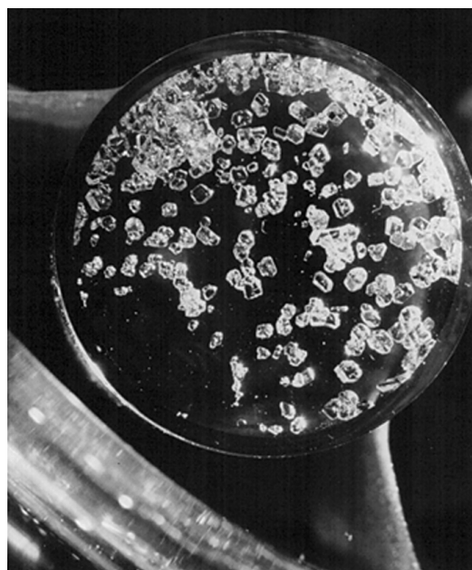
Figure K.4 Xenon tetrafluoride crystals. Xenon tetrafluoride was first prepared in 1962 by the direct combination of \text{Xe}(g) and \text{F}_2(g) at 6 bar and 400^\circ\text{C} .
