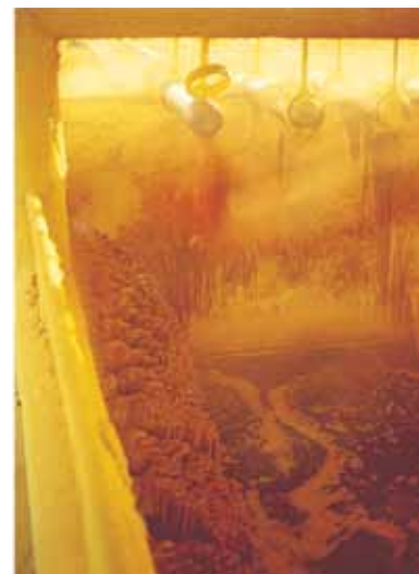
Figure J.3 The Frasch process for sulfur extraction. ( left ) Three concentric pipes are sunk into sulfur-bearing calcite rock. Water at 180°C and 7 bar is forced down the outermost pipe to melt the sulfur. Hot compressed air is forced down the innermost pipe and mixes with the molten sulfur to form a foam of water, air, and sulfur. The mixture rises to the surface through the middle pipe. The sulfur, when dried, has a purity of 99.5%. ( above ) Sulfur with hot water and air can be seen surfacing from Culberson Mine in West Texas.
