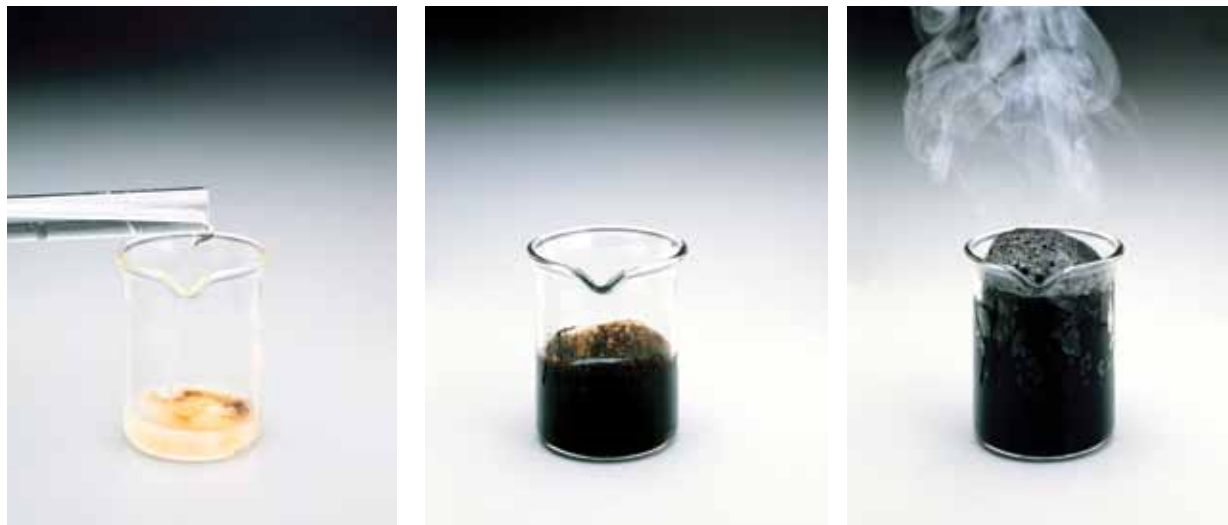
Figure J.11 Concentrated sulfuric acid is a powerful dehydrating agent capable of converting sucrose to carbon.
