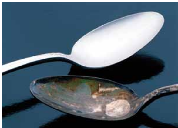
Figure J.13 Silver sulfide is a black, insoluble solid that appears as a dark tarnish on the surface of silver.
