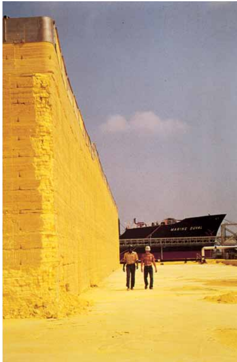
Elemental sulfur occurs in large underground deposits along the Gulf Coast of the United States. The sulfur shown here was mined by the Frasch process and is awaiting shipment at Pennzoil's terminal at Galveston, Texas.
